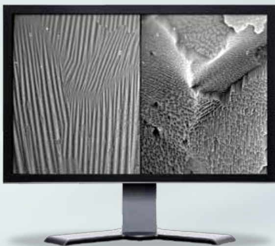
Visualization of domains in electrical steel plates
