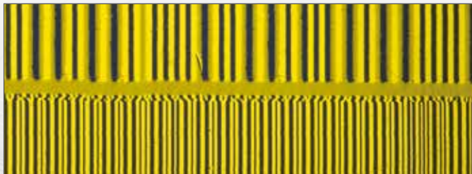
Pictures: visualization of the magnetic Structure of linear encoders
